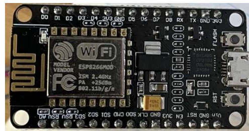
Figure 1 – NodeMCU 12E - notice the WiFi antenna on the left (squiggly line).
