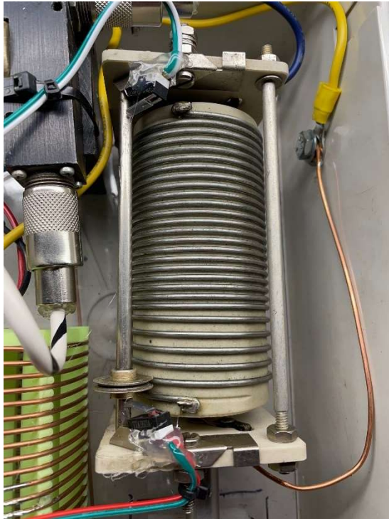
Figure 3 – Close-up of the roller inductor with the end stop switches hot-glued into place. What? It worked.
