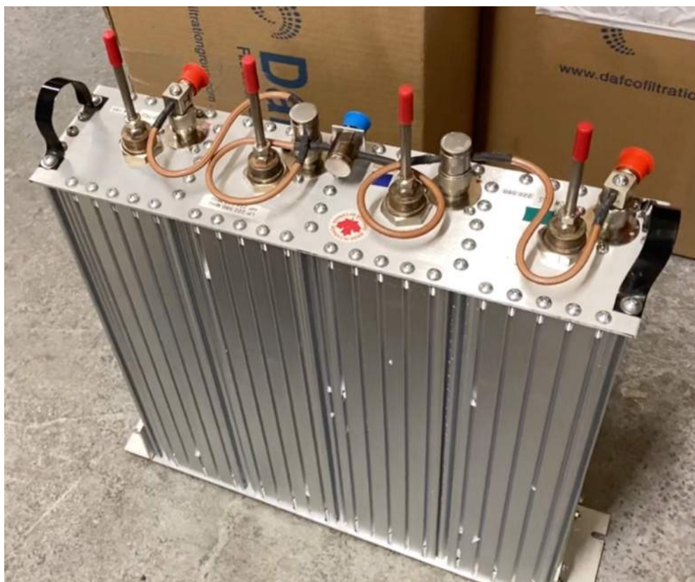
Figure 3: Sinclair Q2221E 4 cavities Duplexer
