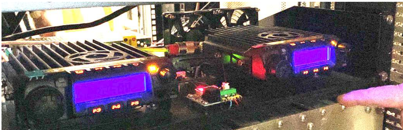
Figure 1: Tytera TYT 9000D 220 Repeater Assembly
