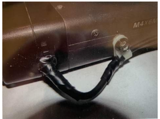
Figure 2—A small nylon clamp holds the microphone cord in place. The clamp is held by one of the screws used in the mobile mounting bracket.
