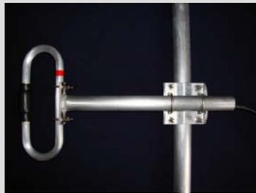
1/2 - wave spacing (3 - 3.7 dBd gain) (Bi-directional / Elliptical pattern)
